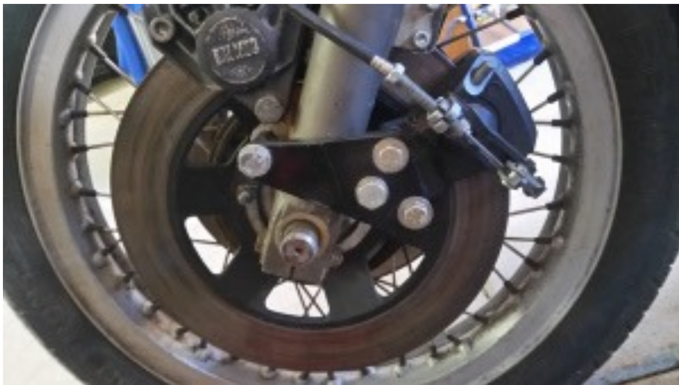
The cable-operated disk brake is clamped to the left fork lower, mounted behind the fork leg.
