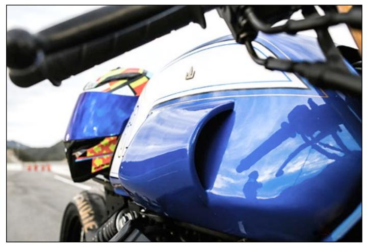
over the top now extending out over the valve covers. The back section of the tank was smoothed out to fill some of the lines that are normally taken up by the stock seat.
