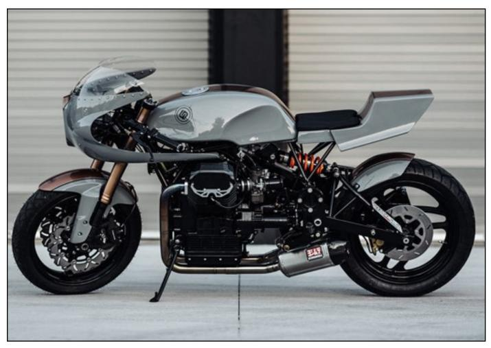
The brakes are from a newer GSX-R, upgraded with aftermarket rotors. Adam also installed a new shock from Matris out back, but left the stock Guzzi rear wheel in place. (We reckon it's a great visual match for the Suzuki front).
